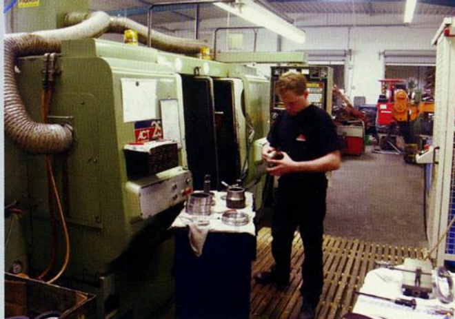
This twin-spindle horizontal lathe was successfully converted to dry machining
